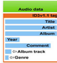
Figure 6. ID3 Tag Structure
