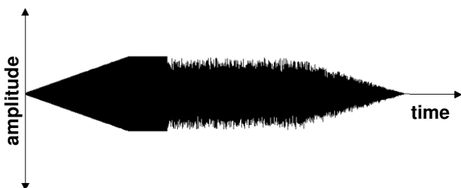
Figure 3: Waveform of test signal. The first portion consists of three harmonically related partials. The second portion is broad band noise.
