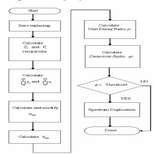
Figure 7: The flow chart of audio bandwidth extension.
