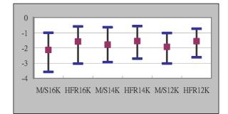
Figure 18: The ODG range of the mp3 with M/S coding and H.F.R audio with different cut-off frequencies under 96k bit rate.
