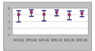
Figure 14: The ODG range of the mp3 with M/S coding and H.F.R audio with different cut-off frequencies under 128k bit rate.
