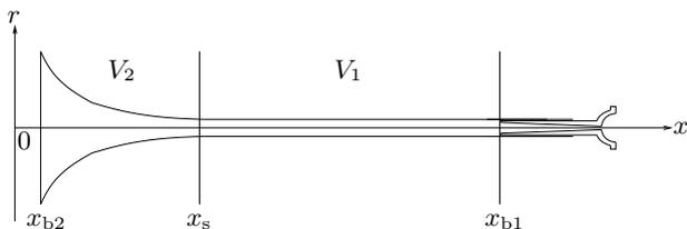
Figure 2: Profile of a brass instrument. Details of the shape vary with the instrument. At the coordinate  $x_{b1}$  the air column is connected to the mouthpiece.  $x_{b2}$  is the coordinate of the bell's end. The cylindrical and the horn shaped part are connected at  $x_s$ .
