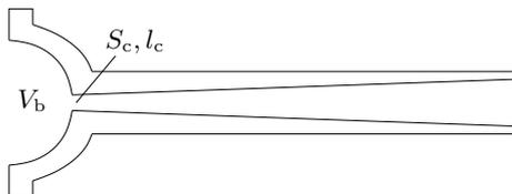
Figure 3: Profile of a typical brass instrument mouthpiece
