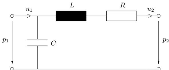
Figure 4: Analogous acoustic network for a brass mouthpiece.
