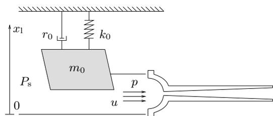
Figure 5: Schematic of a physical model for the lips of a brass player according to [6].
