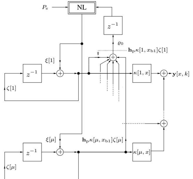
Figure 6: Synthesis algorithm for brass instruments. Simulation of the air column is performed with several complex 1st-order resonators in parallel. The excitation is computed with a nonlinear loop back containing mouthpiece and lip model computations.
