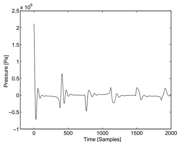
Figure 7: Impulse response of a brass instrument simulated at a sampling rate of 44100 kHz. The parameters of the model are adjusted to fit the measures of a trumpet.
