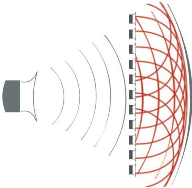
Figure 1: Principle of WFS: Superposition of secondary sound source recreates sound-field
