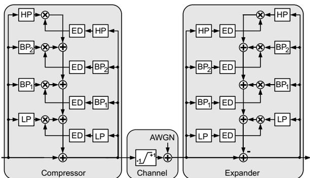
Figure 17: Block diagram of the digitally implemented feedback multi-band additive compander emulation. HP/LP/BP: high/low/band-pass, ED: envelope detection, AWGN: additive white Gaussian noise.
