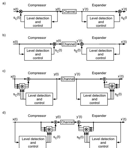
Figure 2: Feed-back and feed-forward control structures of syllable and formant companders. Single-band multiplicative structure with control signal derived a) from the compressed signal and b) from the original signal. Multi-band additive structure with control signal derived from c) the compressed signal and d) from the original signal.
