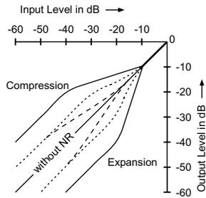
Figure 11: Compression characteristic of Dolby C [3].
