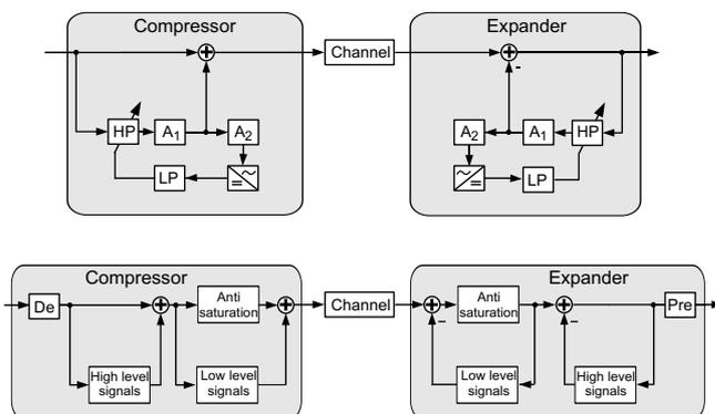
Figure 10: Block diagram of the Dolby B (top) and Dolby C (bottom) compander systems [3].
