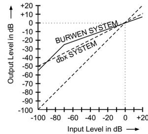
Figure 15: Compression characteristic of the dbx and the Burwen compander [3].
