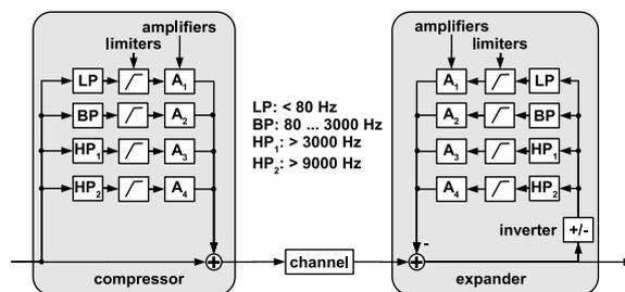
Figure 5: Block diagram of the Doby A compander.
