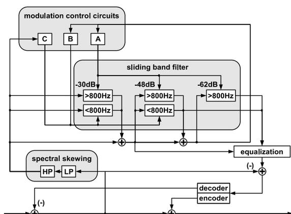
Figure 7: Block diagram of the Dolby SR compander system [3].
