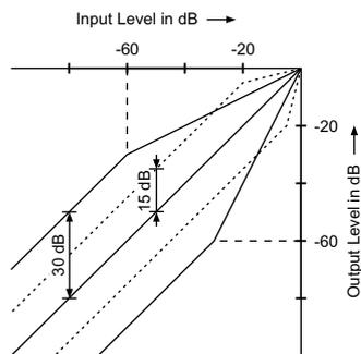
Figure 3: Example compressor and expander laws. Solid line: compression threshold -60 dB, maximum gain 30 dB, compression ratio 2, compression onset 0 dB. Dotted line: compression threshold -20 dB, maximum gain 15 dB, compression ratio 4, compression onset 0 dB.
