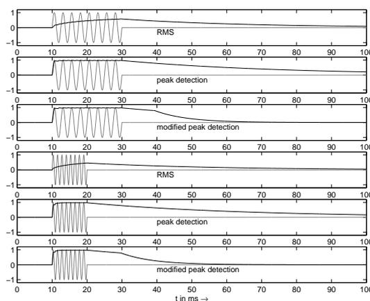
Figure 4: Temporal behavior of different envelope estimates with attack and release time constants.
