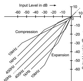
Figure 9: Compression characteristic of the TELEFUNKEN Telecom C4 compander system [3].
