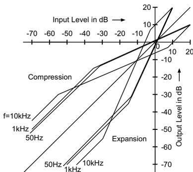
Figure 13: Compression characteristic of HighCOM [3].
