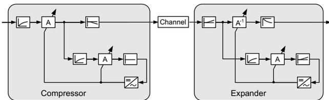
Figure 12: Block diagram of the TELEFUNKEN HighCOM single-band consumer version of the professional Telcom C4 system [3].
