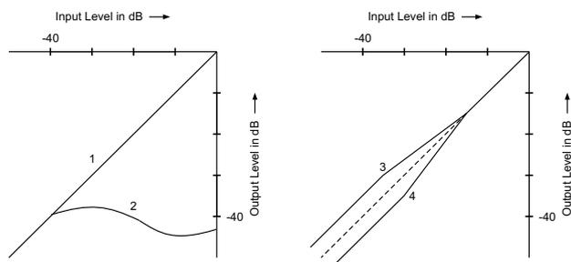
Figure 6: Compression characteristic of Dolby A. Curve 2: characteristic of the control signal added to the direct path. This results in the compression (3) and expansion (4) characteristics.
