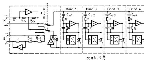
Figure 8: Block diagram of the TELEFUNKEN Telecom C4 compander system [3].
