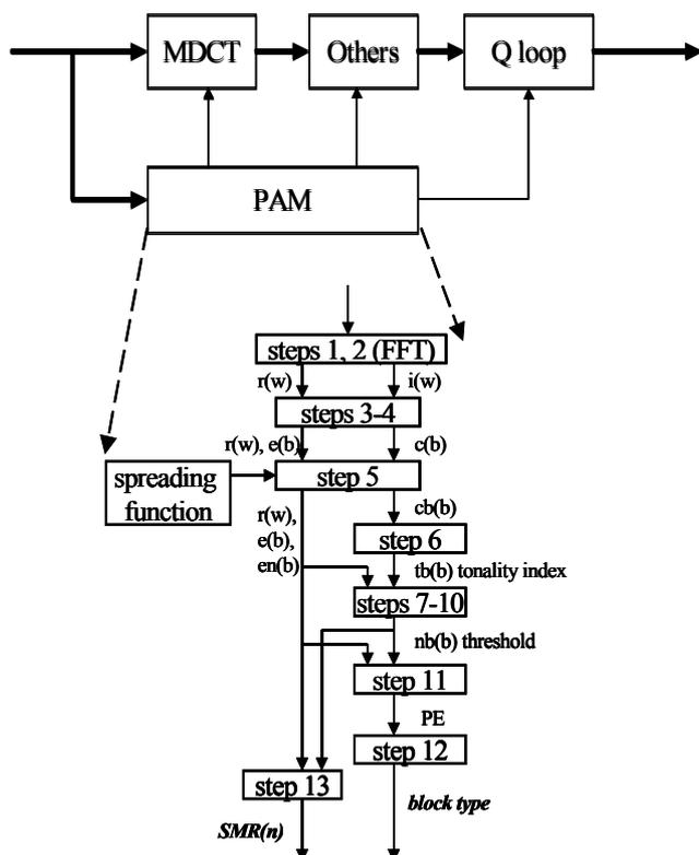
Figure 1: The spreading function of psychoacoustic model in an AAC encoder.
