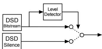
Figure 5: A hard noise gate implemented on a DSD bitstream. A DSD silence signal must be used since constant DC levels are not possible.
