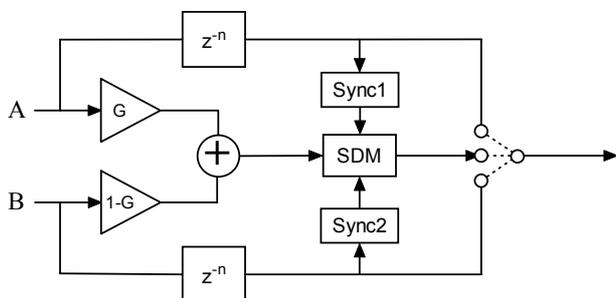
Figure 6: Smooth switching between bitstreams using synchronisation.
