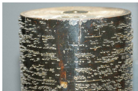
Figure 1: Detail of a typical mechanical organ cylinder.
