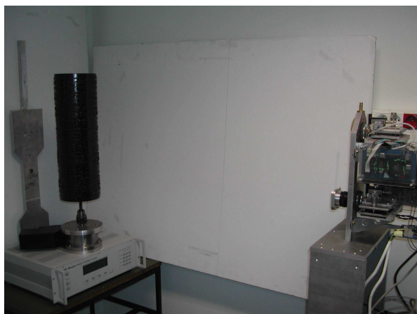
Figure 2: Picture of the experimental setup. On the left: the cylinder on the step-by-step motor and its command box, on the right: the camera with its controller interface.
