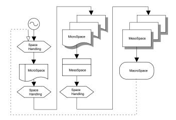
Figure 3: This is the schematic overview of the audio routing and the event space organization inside the application. The audio enters top-left. The dotted line is the feedback line.
