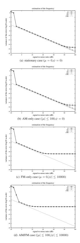
Figure 5: Frequency estimation error as a function of the SNR (stationary, AM-only, FM-only, and AM/FM cases) for the R, ED, and TD methods, and comparison to  $CRB_{\omega}$ .
