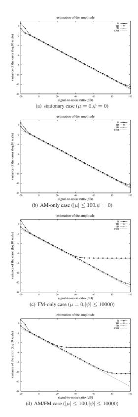
Figure 2: Amplitude estimation error as a function of the SNR (stationary, AM-only, FM-only, and AM/FM cases) for the R, ED, and TD methods, and comparison to  $CRB_a$ .
