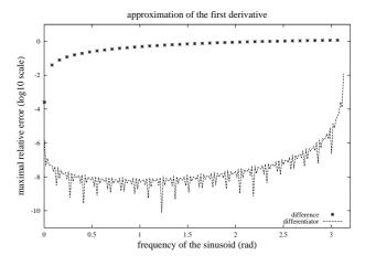
Figure 1: Maximal estimation error when approximating the (first) derivative of a sinusoid using the order-1023 differentiator. The error is acceptable for all but very high frequencies. As a comparison, the error obtained with the classic difference approximation (equivalent to choosing  $\epsilon = 1/F_s$  in the expression of Equation (23)) is plotted with stars \*.
