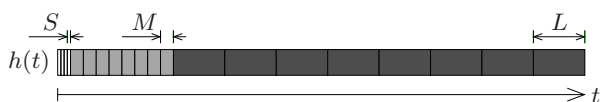
Figure 7: Segmentation of the impulse response h(t) for a convolution with three segment lengths
