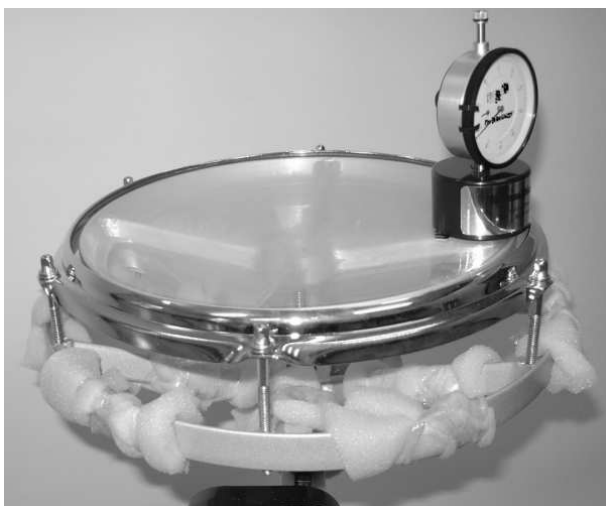
Figure 2: Recording setup: the rototom is tuned with a precision drum tuner, and the support is damped with foam.
