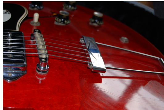
Figure 2: The bridge and tailpiece in a Gibson ES335 semiacoustic guitar.
