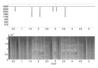
Figure 3: Adaptive analysis with a mask privileging frequencies below 300Hz, on a music signal with a bass guitar, a drum set and a female singing voice starting from second 1.54: on top, best window size chosen as a function of time; at the bottom, adapted spectrogram of the analyzed sound file.
