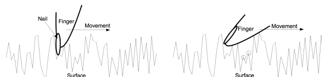
Figure 3: Left: A nail which is scratching a surface. Right: A finger which is rubbing a surface (asperities which are not "seen" by the finger are circled). For clarity, dimensions of the asperities are exaggerated on the scheme.
