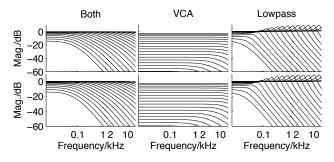
Figure 5: Magnitude response of modes of digital models of LPG circuit, for values of  $R_f$  between  $1k\Omega$  and  $1M\Omega$ . Top: DF2T model. Bottom: Topology-preserving model.
