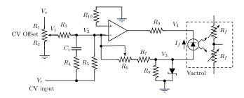
Figure 7: Simplified schematic of the Buchla 292 control path.
