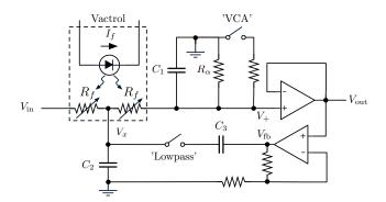
Figure 1: Simplified schematic of the Buchla 292 LPG audio path.
