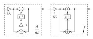
Figure 4: Block diagrams of direct form II transposed (DF2T) integrator and differentiator elements.
