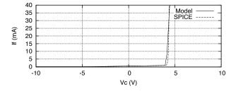
Figure 8:  $V_c$  to  $I_f$  relations, produced by model and by SPICE.
