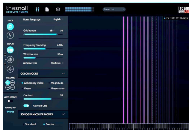
Figure 8: Sonogram in its precise mode: compared to figure 7, only the (colored) refined part are displayed. This mode exactly mirrors the visual representation in the snail display.
