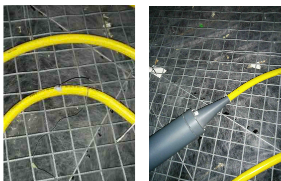
(a) Microphone inside the tube with gray moldable plastic to attach it to the hole. (b) Loudspeaker attached to the end of the tube with a conical adaptor.
