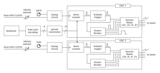
Figure 2: Overview of the Welson Syntex sawtooth generation mechanism.
