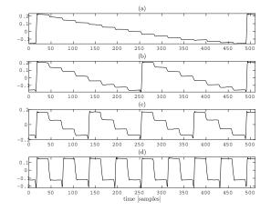
Figure 5: The four sawtooth waveforms sampled from the instrument output with the VCF completely open: 32' (a) to 4' (d). The effect of the sound card DC blocking stage affects the waveform shape by tilting the steps, while some light lowpass filtering due to parasitic components in the analog path slightly smooths the waveforms. This is not seen using an oscilloscope directly at the output of the components.
