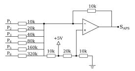
Figure 6: Sawtooth waveform generation in the ARP Pro Soloist. The input square wave signals  $P_1, ..., P_6$  are generated by a top octave divider.  $P_1$  is the lowest generated octave, corresponding to the note fundamental.
