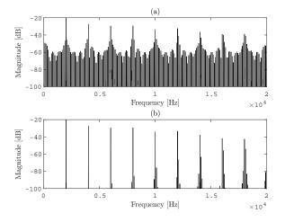
Figure 8: Magnitude spectrum of a 2 kHz  $S_4$  signal generated at 44100 Hz without aliasing suppression (a) and with 4-samples BLEP (b) according to emulation option B.
