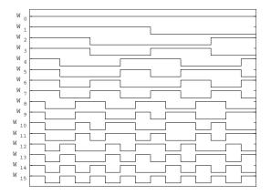
Figure 1: Walsh matrix of order M = 16, plotted row-wise. The signals constitute orthogonal bases that are employed in the Walsh transform. The first line corresponds to Walsh function of order 0 (DC), or  $W_0$ , while the last has index M - 1.
