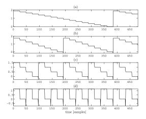
Figure 4: Simulation of the four sawtooth waves from the Welson oscillator: 32' (a) to 4' (d). The duty cycle of the Q signal has been set to 1%.
