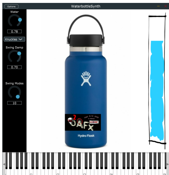
Figure 11: Real-time modal synthesizer model of the HydroFlask 32 oz. Wide Mouth.
