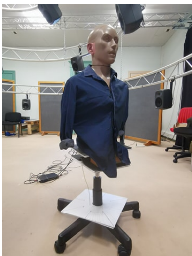
Figure 7: Experimental recording setup with the KEMAR manikin. The manikin was moved into the space intended for listeners in order to produce the cartography
