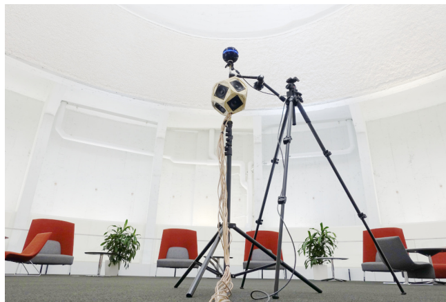
(b) Loudspeaker with one Ambisonic microphone used during measurements at the Centech.
