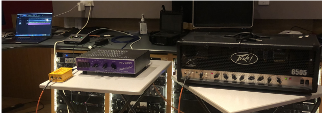
Figure 2: Equipment setup for the recording of the amplifier output.
